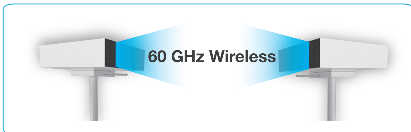
Figure A mmWave Wireless Backhaul Concept
