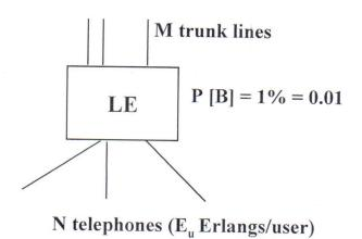
Question 2: For a N x N LE {actually (N + M) x (N + M) with M trunk lines}, how many cross-points are required for a 1% blocking switch?
