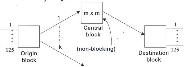
With n = 125, generated traffic for the block = 125  $E_u$ This gets divided (equally) between the k = 10 lines
