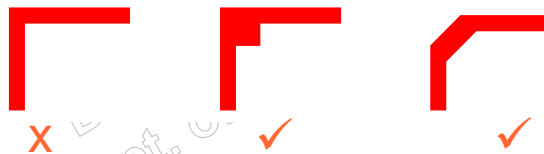
Bending of a high current line
